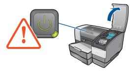
2 Remove the ink cartridge that requires replacement by grasping it between your thumb and forefinger and pulling it firmly toward you.
